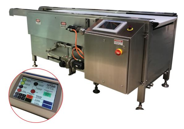
The KOFAB Retractor signature design can be used for an array of applications including transposing product from a wide to narrow pattern, pan loading, oven and freezer belt loading, or for simpler applications such as rejects or product dumps.
